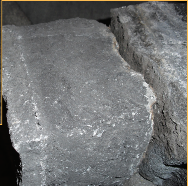
LadleMag sintered onto working brick
